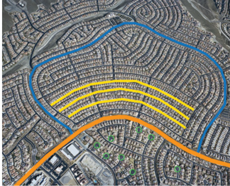
Figure 9: Diagram of street types. Arterial streets (orange), collector streets (blue), local streets (yellow), and cul-de-sacs (greens). Photo credit: dailymail.co.uk . Annotations by the author.
